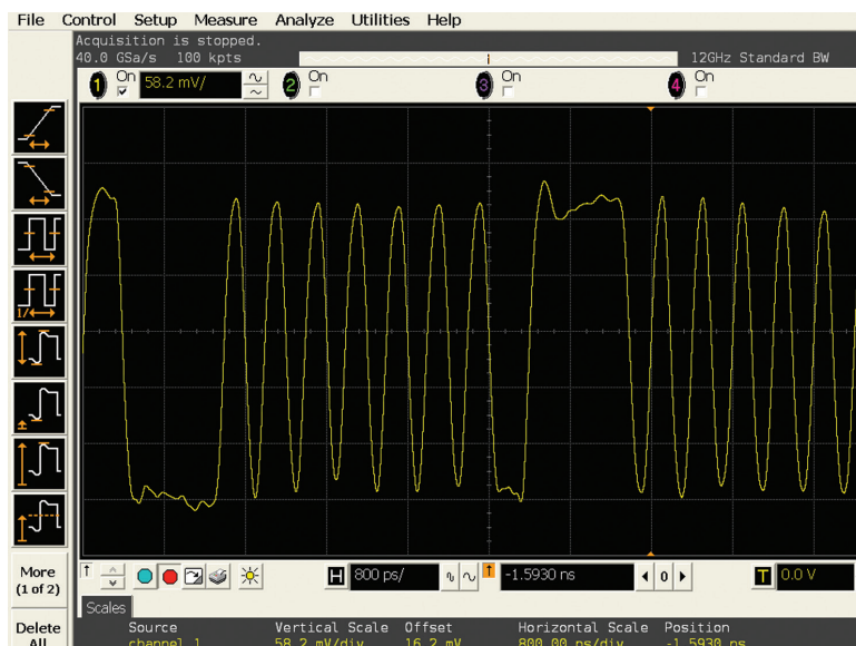
Figure 1. PCI Express 2.0 supports data rates up to 5.0 GT/s as shown above (-3.5 dB de-emphasis)
