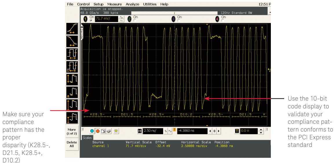
Figure 24. The 8b/10b decoded symbol information is shown below the appropriate portion of a PCI Express signal using the E2688A software.
